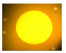
Top View of Circulator Chip after Etching SiO<sub>2</sub> Operational in 10 GHz -100 GHz Range
